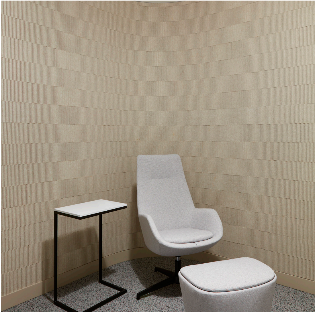
Acoustical PET wall covering with a ribbed texture.
